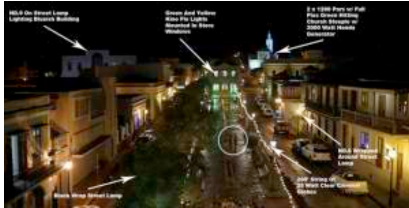
Image 2: VR Film Lighting Setup
