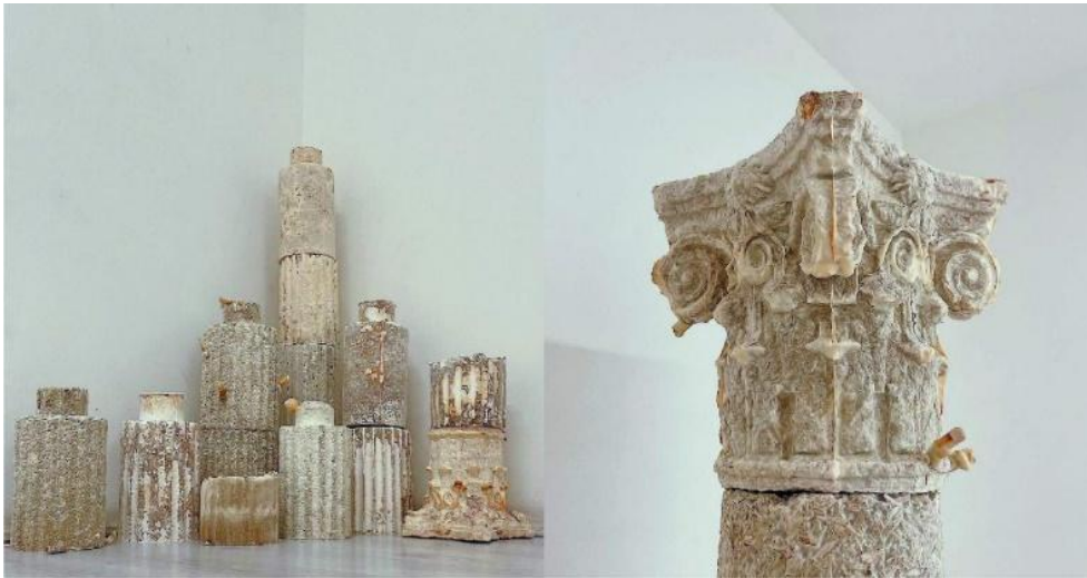
Figure 5 Mycelium columns, mycelium substrate with wood chips
