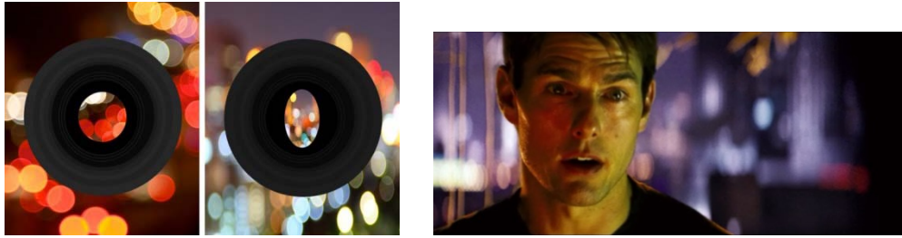
Figure 26: Left Spherical lens bokeh center: Anamorphic lens. Right: Still from Mission Impossible 3, shot with anamorphic lens.
