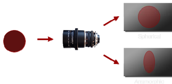
Figure 25: 46 Difference between the Spherical lens and Anamorphic lens, the image that is projected on the spherical does not have changes while (Above) the anamorphic (bottom) is compressed in the horizontal field.
