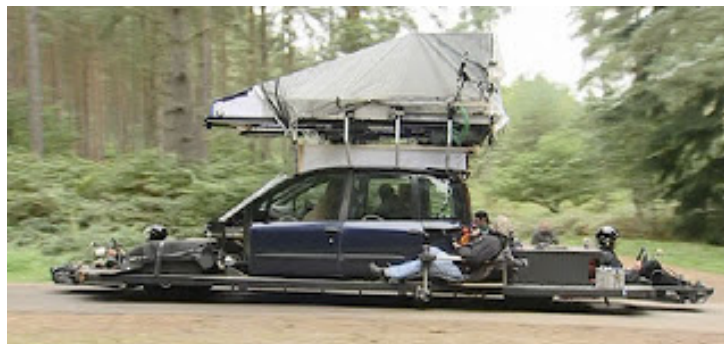
Figure 4.3 Doggicam system was created for the car scene in " Children of men (2006)". 49
